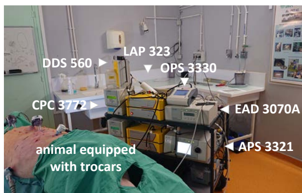
Figure: Photographic image of the two-sectional aerosol-analytical setup for the characterisation of surgical smoke formation and elimination.
